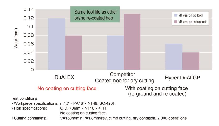
DuAl EX Hob without coating on cutting face after re-grinding has same tool life as other brand Hob after re-grinding and re-coating.
